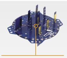
A state-of-the-art smart antenna array integrates six high-gain vertically polarized and six hortizontally polarized antenna elements. This enables up to 4096 potential antenna combinations and up to 7 dBi gain thereby delivering unprecedented range extension and Wi-Fi signal reliability. Expert control software selects the best antenna elements to use at any given moment for any given packet and any given client based on changing environmental conditions
